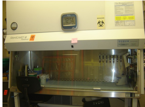
Photo #2 - Biosafety Cabinet - View 1
